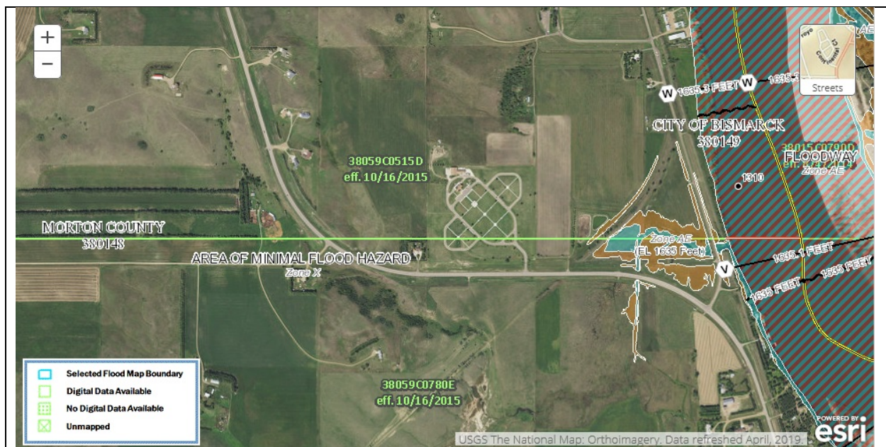
Figure 3.4: Overview of Floodplains Information at the North Dakota Veterans Cemetery and Surrounding Area. The entire area of the NDVC is located in Zone X, area of minimal flood hazard.
