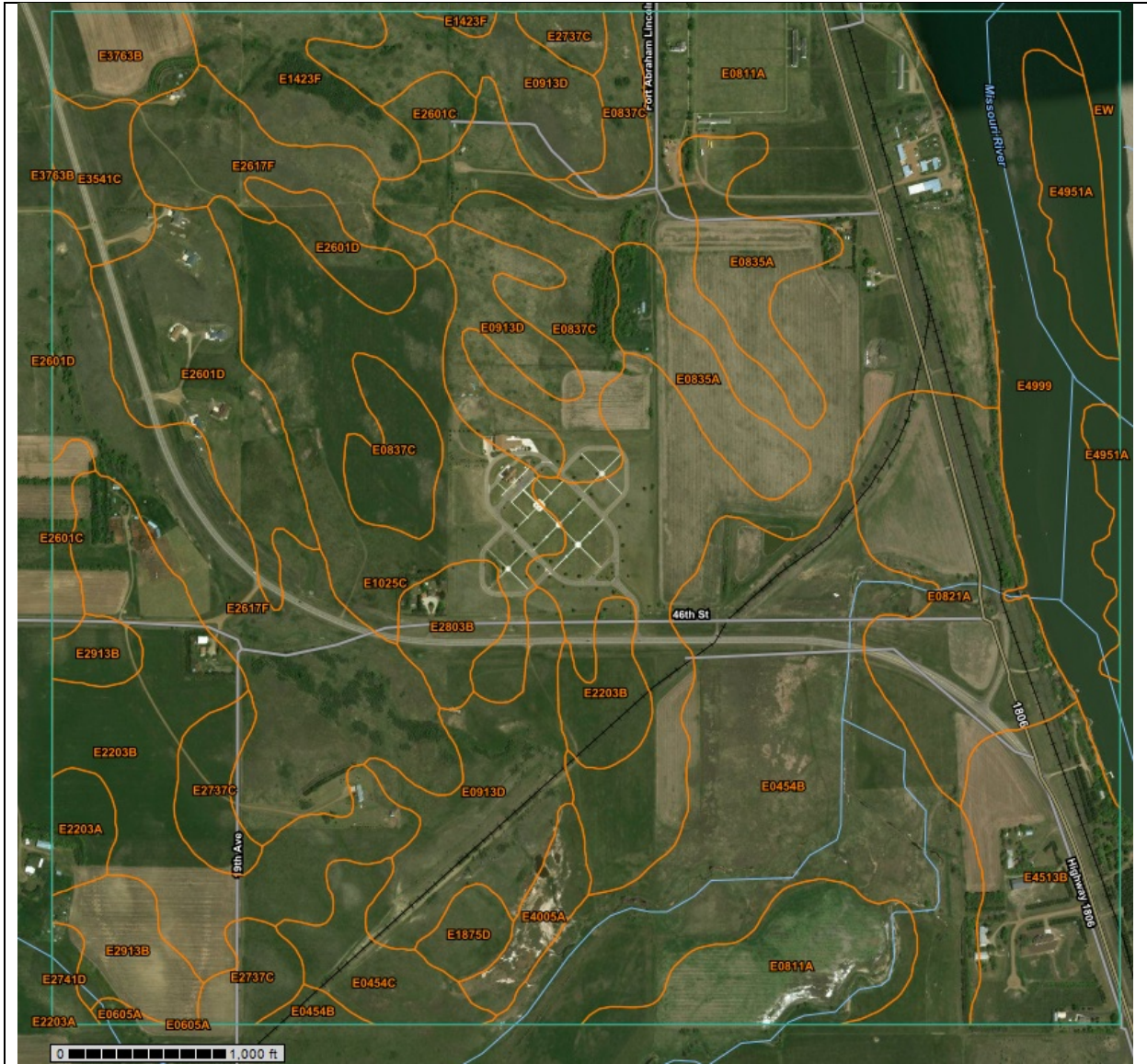
Figure 3.3: Soil Survey Map of North Dakota Veterans Cemetery and Surrounding Area. Within the NDVC there are eight soil types recorded.
